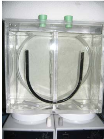
Figure 1. Experimental setup of the conductivity experiment: a u-shaped tube filled with sediment is placed in a water filled Plexiglas box which is divided into two chambers; both chambers are stirred continuously; a Tygon tube ensures the reflux of water to avoid water level differences; in one chamber chloride concentrations are enriched and in the other chamber the increase of chloride concentrations due to chironomid activity is measured with a conductivity electrode (not shown).
