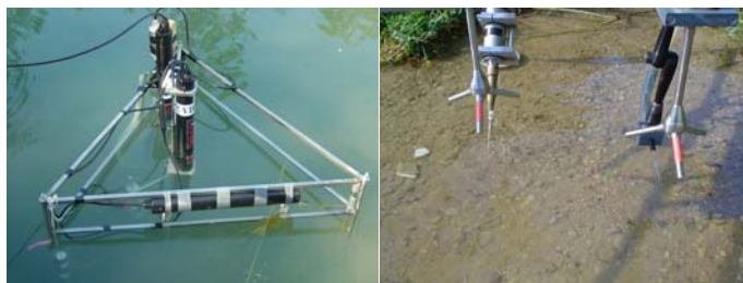
Figure 1: (Left) The two eddy correlation systems mounted next to each other in the measurement site. (Right) A close up of the two systems.
