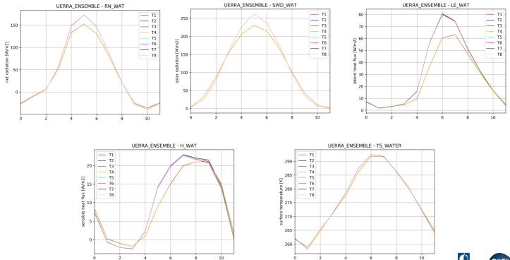
Small sensitivity to 2m air temperature and humidity. Main driver is radiation
