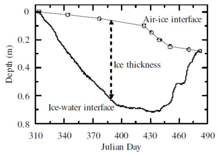
The observed lake ice thickness evolution over the whole 2010/2011 ice season. The open circles denote the observed surface depths, and the solid lines connecting the circles are based on linear interpolation.
